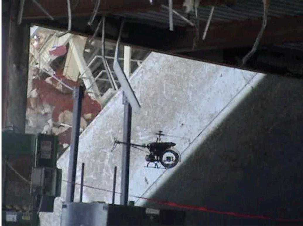
Figure 20: The IP3 flying into a building to image concealed damage.
