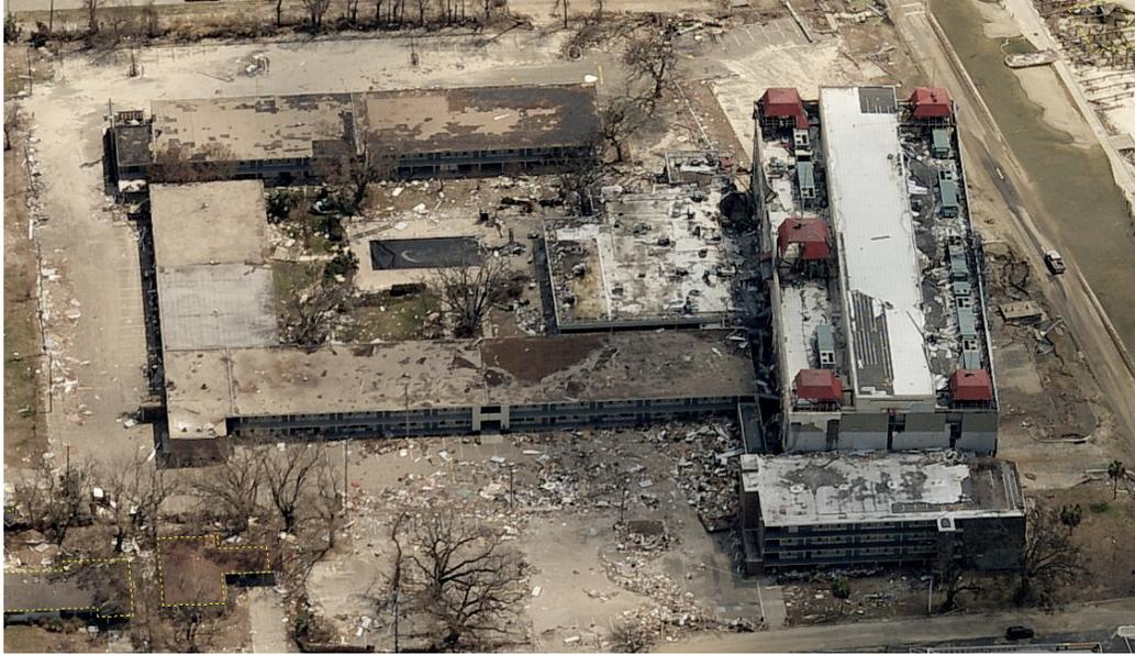
Figure 15: The President Casino barge where it came to rest approximately 1 km down the beach from its original mooring. The barge is the structure on the right of the frame topped by the red towers. The remaining buildings are part of Motel 6. Image is © Hancock County EOC, 2005 and is used with permission.
