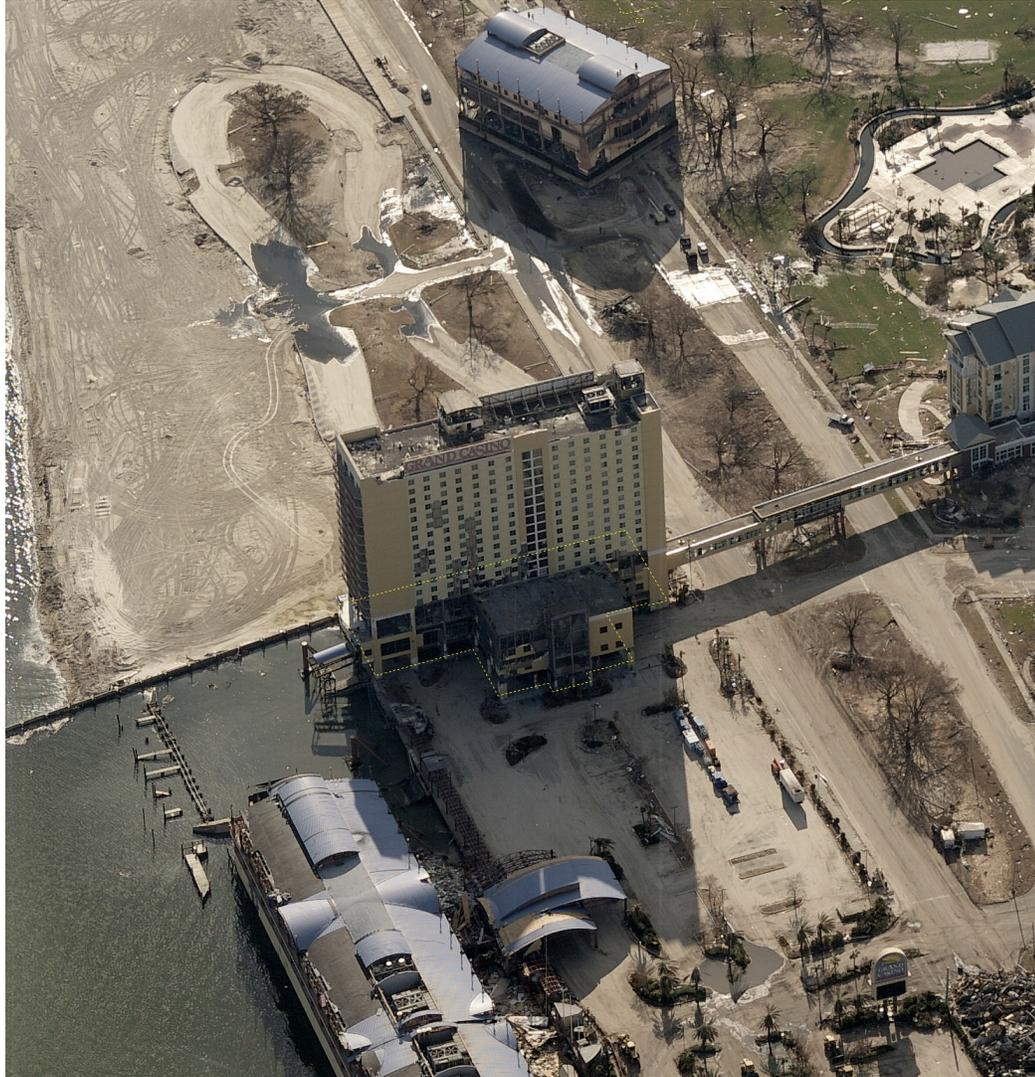
Figure 9: Overhead pictometry of the Gulfport Grand Casino. The blue-roofed barge which is missing from in front of the Grand can be seen near the top of the frame. This was an unfortunately common occurrence up and down the beach. Image is © Hancock County EOC, 2005 and is used with permission.
