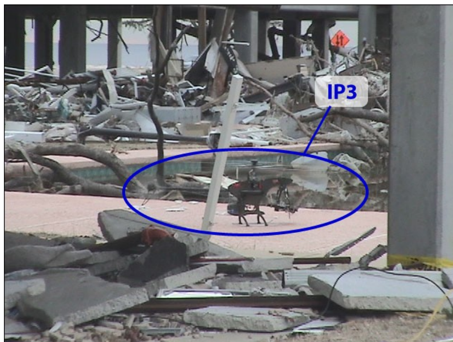
Figure 8: IP3 Launching from a cluttered pool deck. In a disaster area, physical access is often not ideal.
