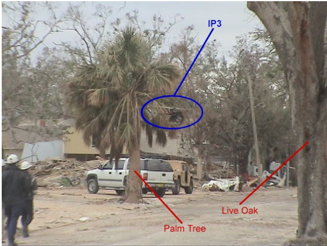
Figure 6: IP3 flying under trees. Here the helicopter is being transitioned from one building face to another. Just out of frame is the canopy of the live oak, which was a large navigation hazard
